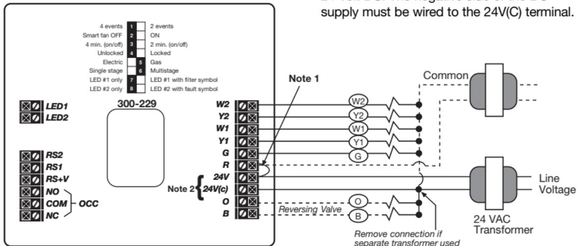
**Note 1:** If jumper is removed, a separate transformer must be used to power the loads.
