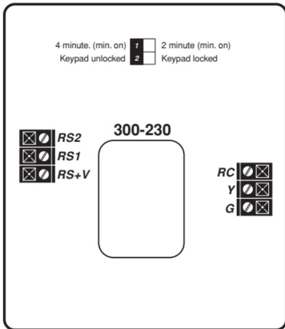
**RC** .....24VAC supply from cooling equipment transformer
